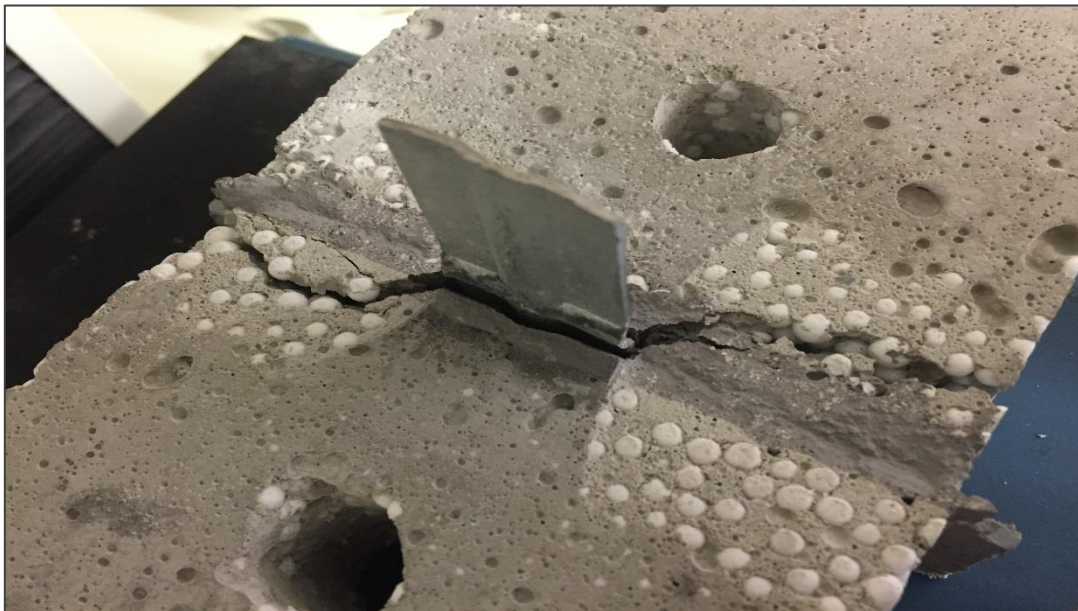
Figure 7: Shear sample - typical failure
