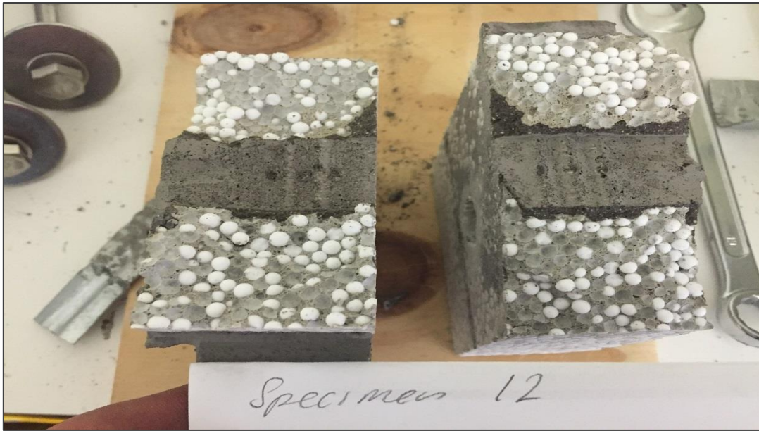
Figure 8: Shear sample - typical failure cross section
