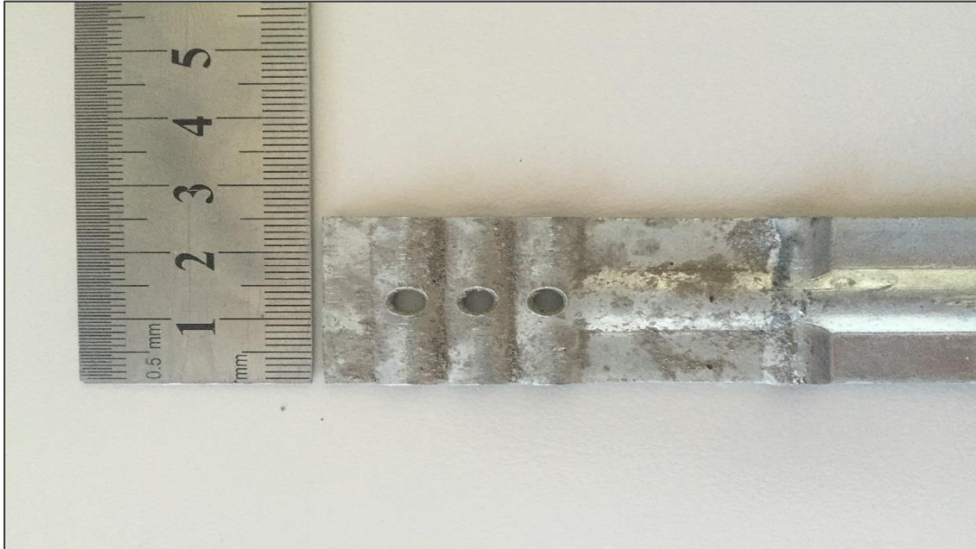
Figure 6: Brick tie - after testing
